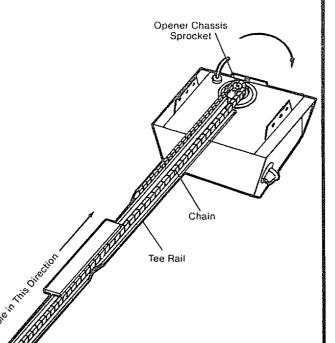
As a permanent trolley stop, insert 5/16" washered screw into remaining hole in Tee rail front. Tighten securely with 5/16" nut. *REMOVETEMPORARYSTOP INSERTED IN STEP 2*.
